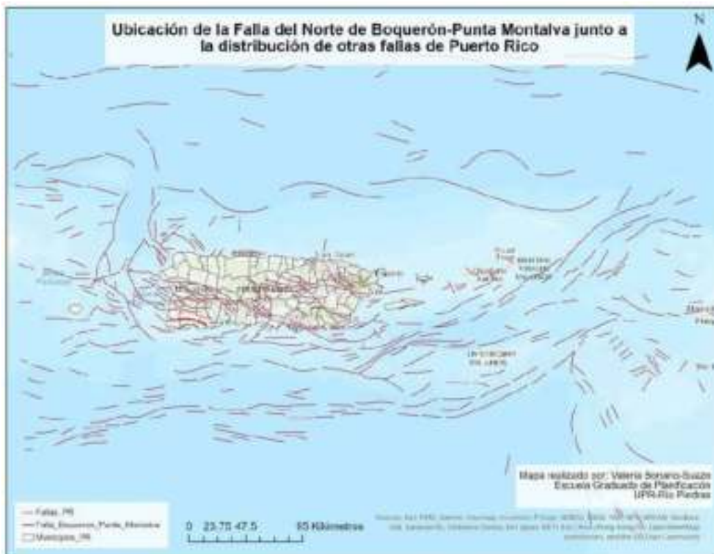
Figure 3-85. Location of the North Boquerón-Punta Montalva fault along with the distribution of other faults.
